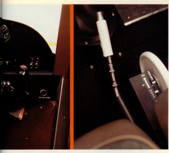
Maule panels are beginning to look high-tech with the options now available from the factory. The flap handle can be set to a negative position, a trick that adds a couple of knots to cruise speed.
